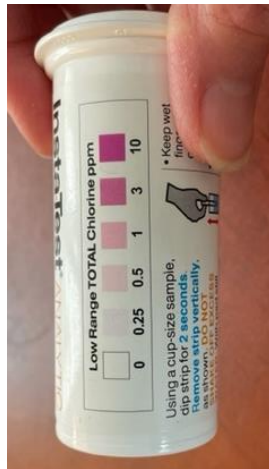
Total Chlorine test strips (0-5 mg/L shown here)
